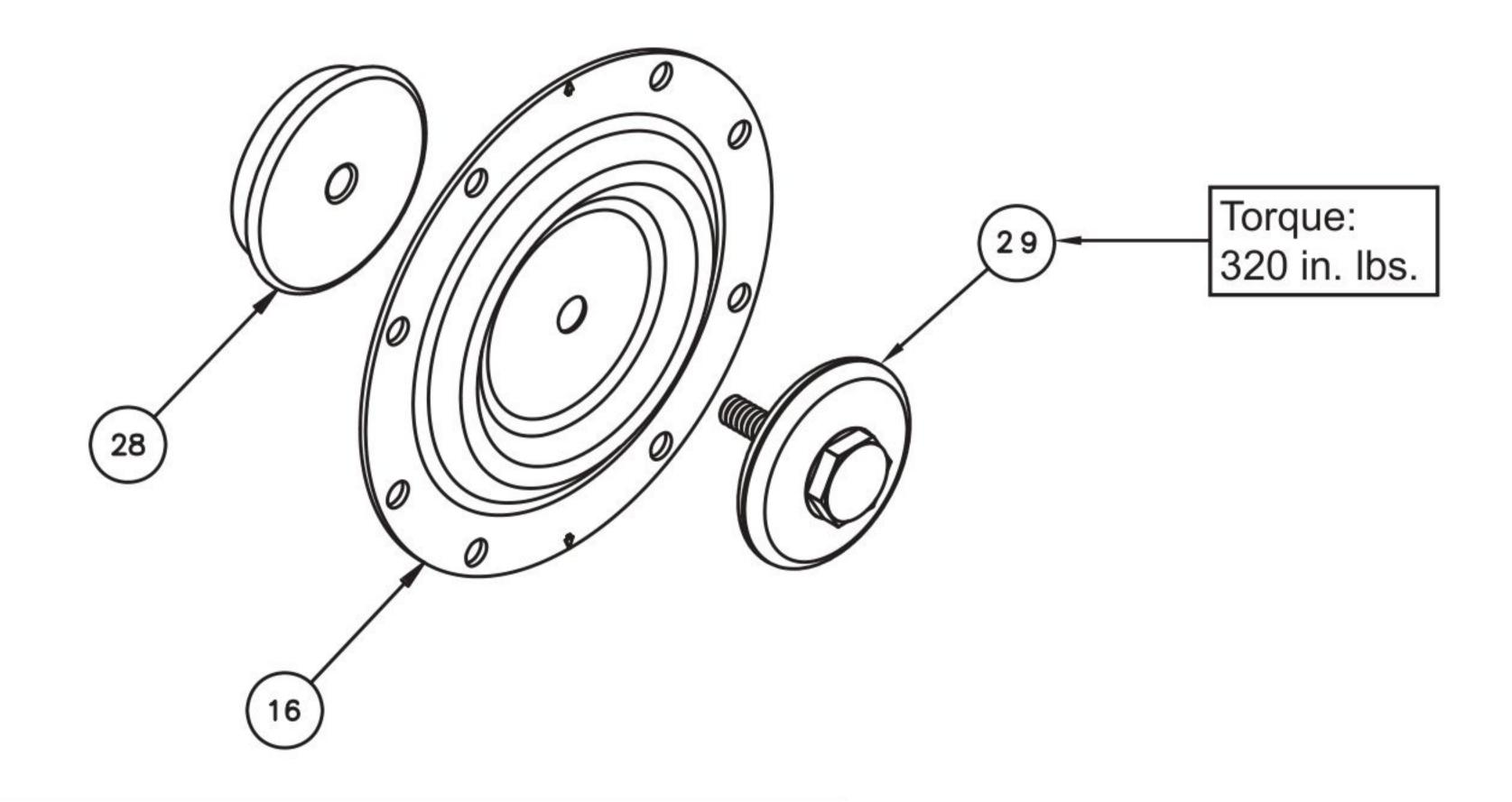
Field conversion kit 475.258.000 available for conversion from PTFE Overlay to One-Piece bonded Diaphragm
